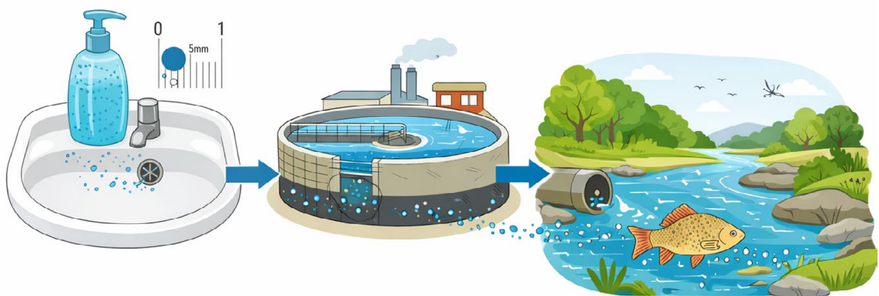
FIGURE 1: Pathway of micropollutants from domestic sources to surface waters
